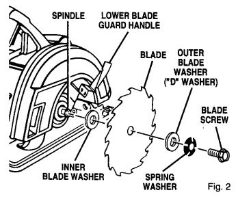
Note: Turn blade screw counterclockwise to remove.
